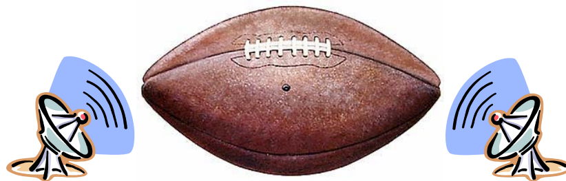
Figure 1. Approximate shape of Fresnel Zone between transmitter and receiver
